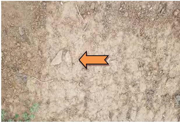
Photo 1. Asbestos-containing fibre cement sheet debris located on the soil surface within Riverwalk Stage 15.
