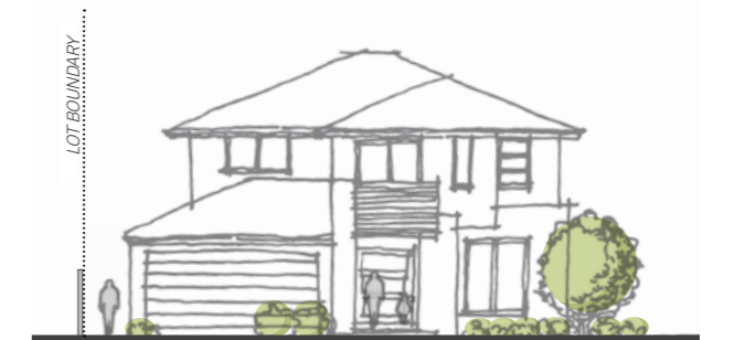
At least 1.0m garage setback from side boundary allows for a path.
