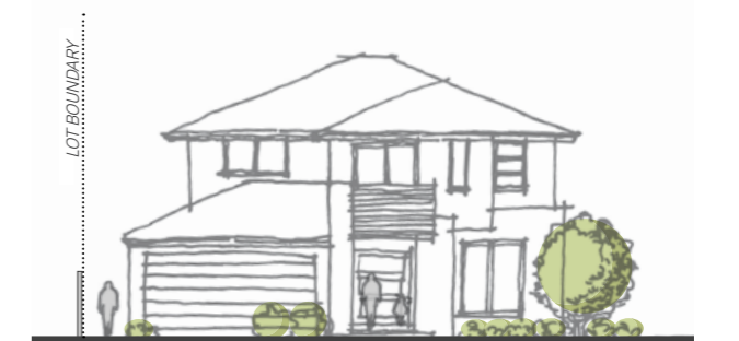
At least 1.0m garage setback from side boundary allows for a path.
